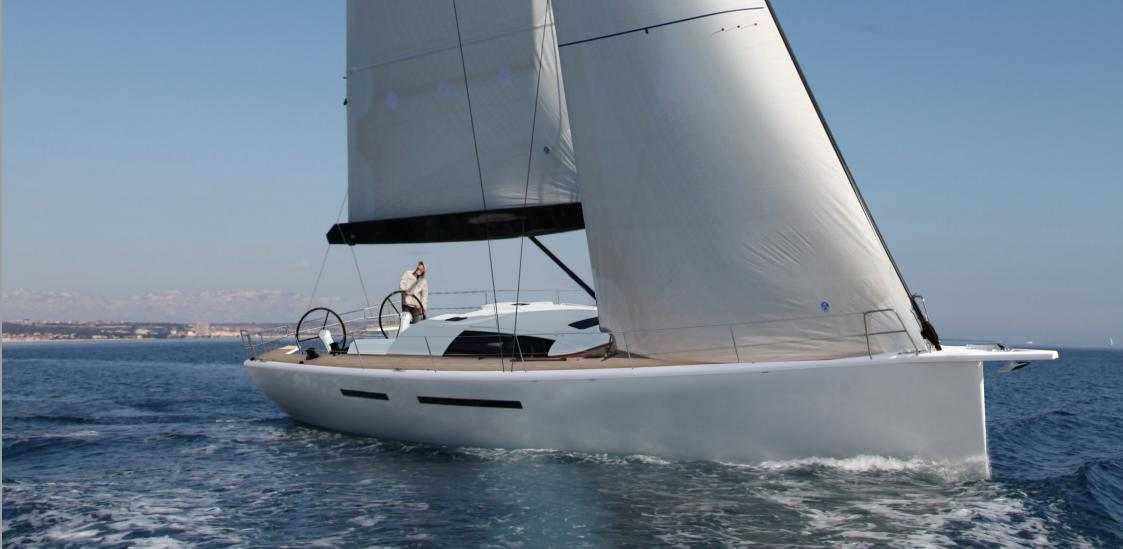
THE MURTIC 52 IRC CARBON HAS BEEN DESIGNED TO DELIVER EXCEPTIONAL PER-FORMANCE IN BOTH RACE AND CRUISING MODES. CONSTRUCTED IN CARBON PRE-PREG, MURTIC 52 IRC CARBON DELIVER EXCEPTIONAL PERFORMANCE RATIO, STA-BILITY AND STRENGHT.
