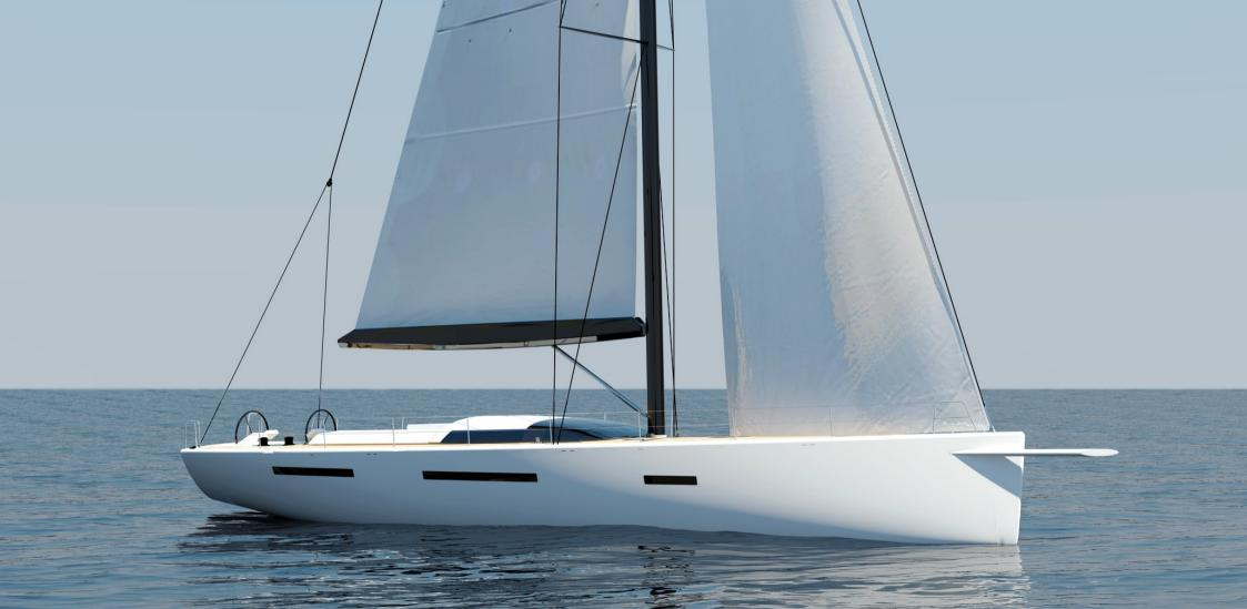
THE MURTIC 67 RS CARBON HAS BEEN DESIGNED TO DELIVER EXCEPTIONAL PER-FORMANCE IN BOTH RACE AND CRUISING MODES. CONSTRUCTED IN CARBON PRE-PREG, MURTIC 67 RS DELIVER EXCEPTIONAL PERFORMANCE RATIO, STABILITY AND STRENGHT.
